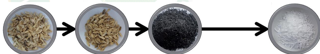
Figure 2 Rice husk before and after calcination.
