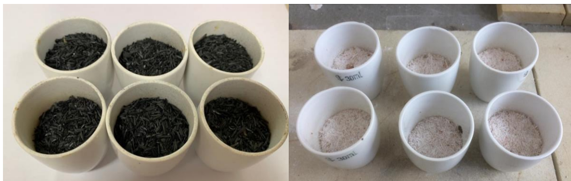
Figure 13 Rice husk before and after calcined.
