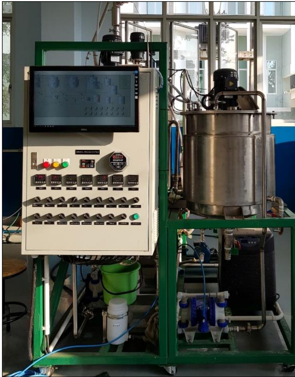
Figure 20 Ethanol production operating system capacity of 150 L per production (AC 400 V 50 Hz; 1.2 m width; 1.7 m length; 1.5 m height and 1,000 kg weight).
