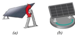
Figure 2 Type single-axis trackers (a) Horizontal and (b) Vertical [9]
