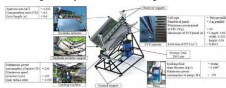
Figure 1. The configuration and characteristics of parabolic concentrating PV/T system.
