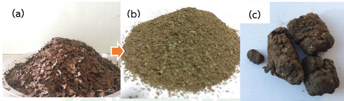
Figure 16 Material Preparation. (a) Dried longan leaves (b) Powdered longan leaves (c) pig manure.
