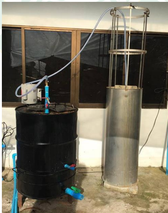
Figure 20 200 L biogas digester system.
