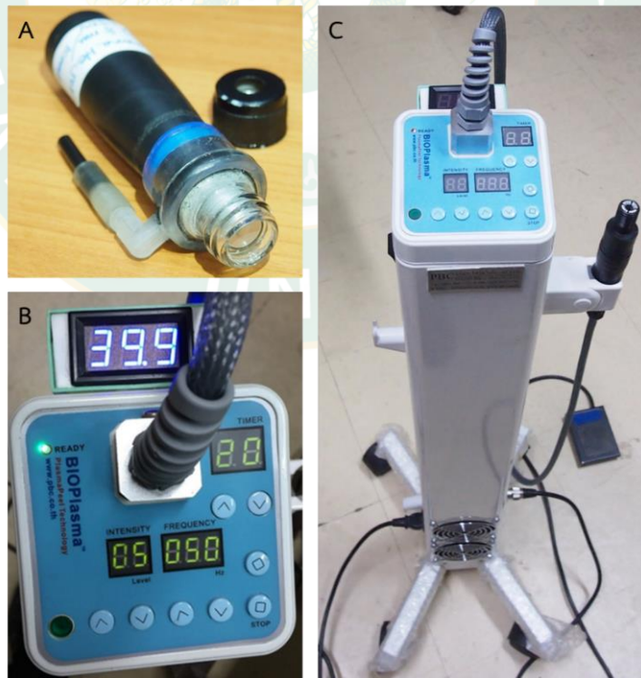
Figure 8 (A) DBDJ, (B) monitor display of power supply and (C) power supply of BIO Plasma.
