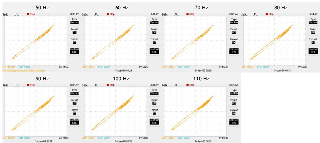
Figure A6 The Lissajous figure of DBDJ at repetition rate 50 Hz to 110 Hz.
